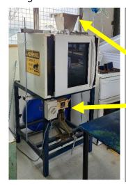
**Photo 1:** Oven positioned sideways with a hopper installed at the top.
