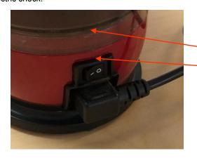
Water was leaking from a small crack in the plastic seam and running down in to the electrical components
