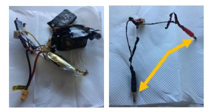
When connecting a device ensure the polarity is around the correct way (i.e. Positive/Red/+ connects to Positive/Red/+ and Negative/Black/- connects to Negative/Black/-)
