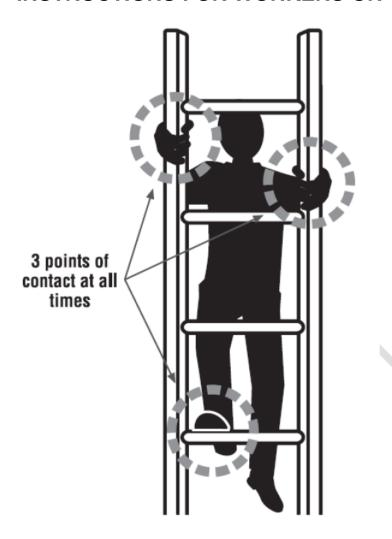
Three points of contact with the ladder should be maintained at all time, i.e. two feet and one hand, two hands and one foot or two fee and the frontal D ring on the harness attached to the arrest/restraint line or inertia reel. Tools and materials should not be carried by hand, They should be in a tool belt or side pouch.
