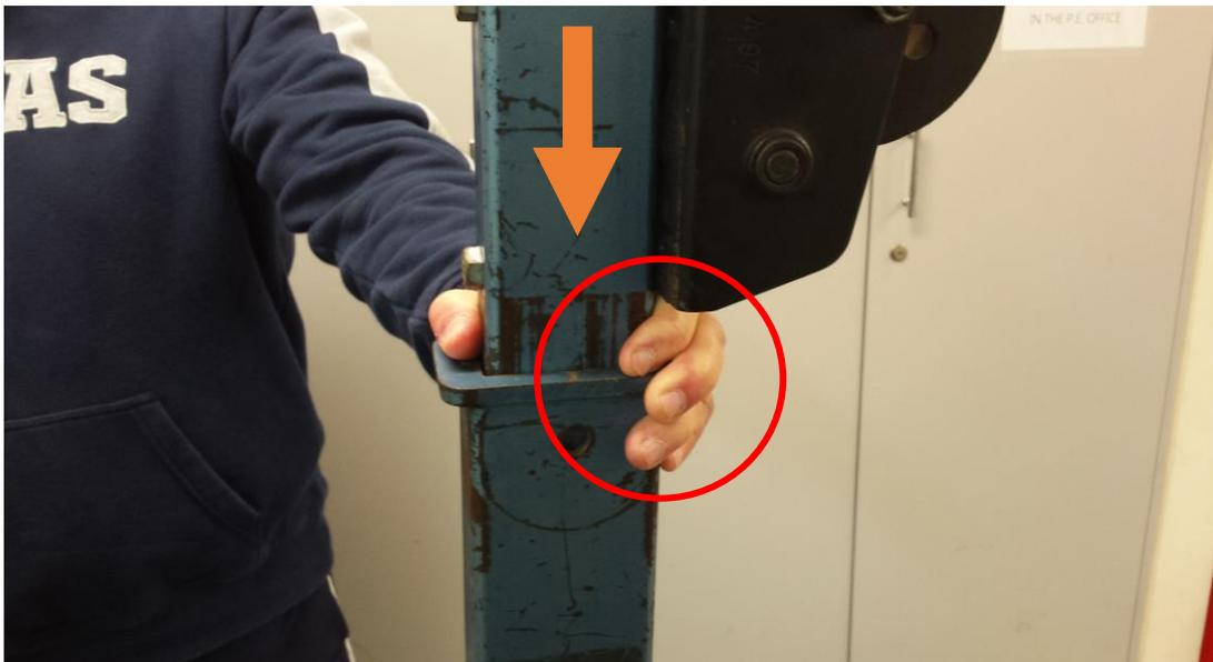
When lifted upright with no pin the top section dropped, crushing the student's finger
