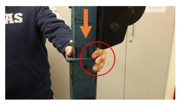
When lifted upright with no pin the top section dropped, crushing the student's finger
